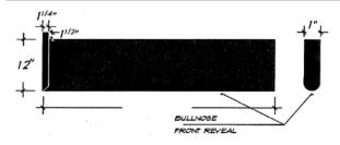
A one end return tread is installed at an open end/sided staircase or stepdown. This tread must be ordered as right hand or left hand, determined by facing the steps from the bottom with the left side or right side needing the return end.
