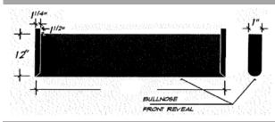
A double end return tread is installed with both ends open requiring a return on both sides. This tread must be ordered with the required inside dimension from each inside edge of the return.
